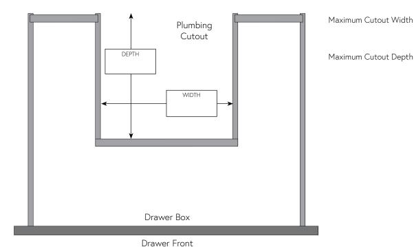
Maximum Opening Width is overall cabinet width minus 8-5/8". This allows for a 4" alley on both sides.
